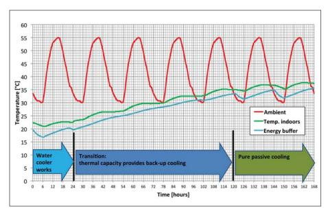
Fig. 4. Testing verified the shelters' intrinsic ability to deal with the failure of active cooling systems.
